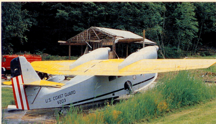
The rugged landing gear allows a Widgeon to be safely taxied up an unimproved lakeside ramp and into the owner's backyard.
