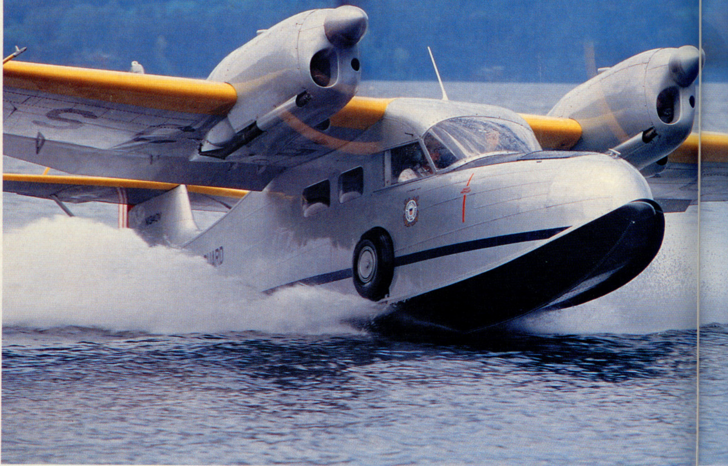
The 200-horsepower inverted in-line Ranger engines are mounted high above the water's surface to prevent spray from damaging the propellers during takeoff.
